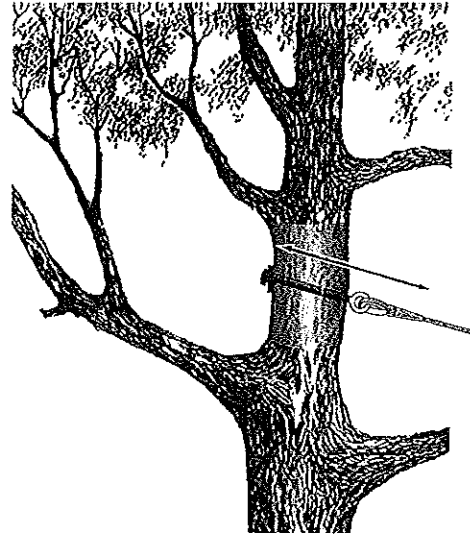
Fig. 33.5.3 Correct cable and hardware alignment
